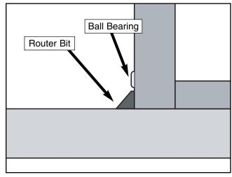
**Figure 24.** Proper setup for profile cutting. (Side View)
